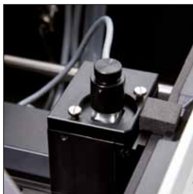
The peltier temperature controlled cell holder guarantees high temperature accuracies; the temperature is measured directly in the cell.
