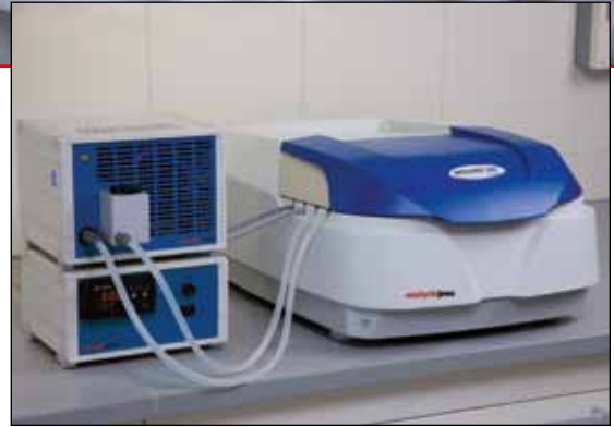
Peltier temperature controlled 8-cell changer performing measurements with high temperature accuracy
