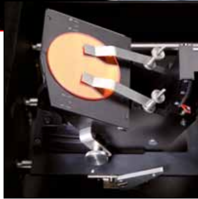
Reflectance attachment with variable angle for determining the refraction index and the film thickness
