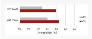
Drinking water analysis according to U.S. EPA 200.8. RSD of certified reference materials were measured with two different speeds. The outstanding sensitivity allows to measure >80 water samples per hour with competitive precision.
